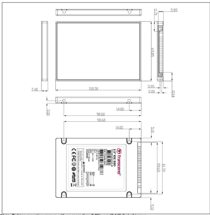
\*Note: Tighten mounting screws with no more than 2.0Kg-cm (0.14ft-lbs) of torque.
